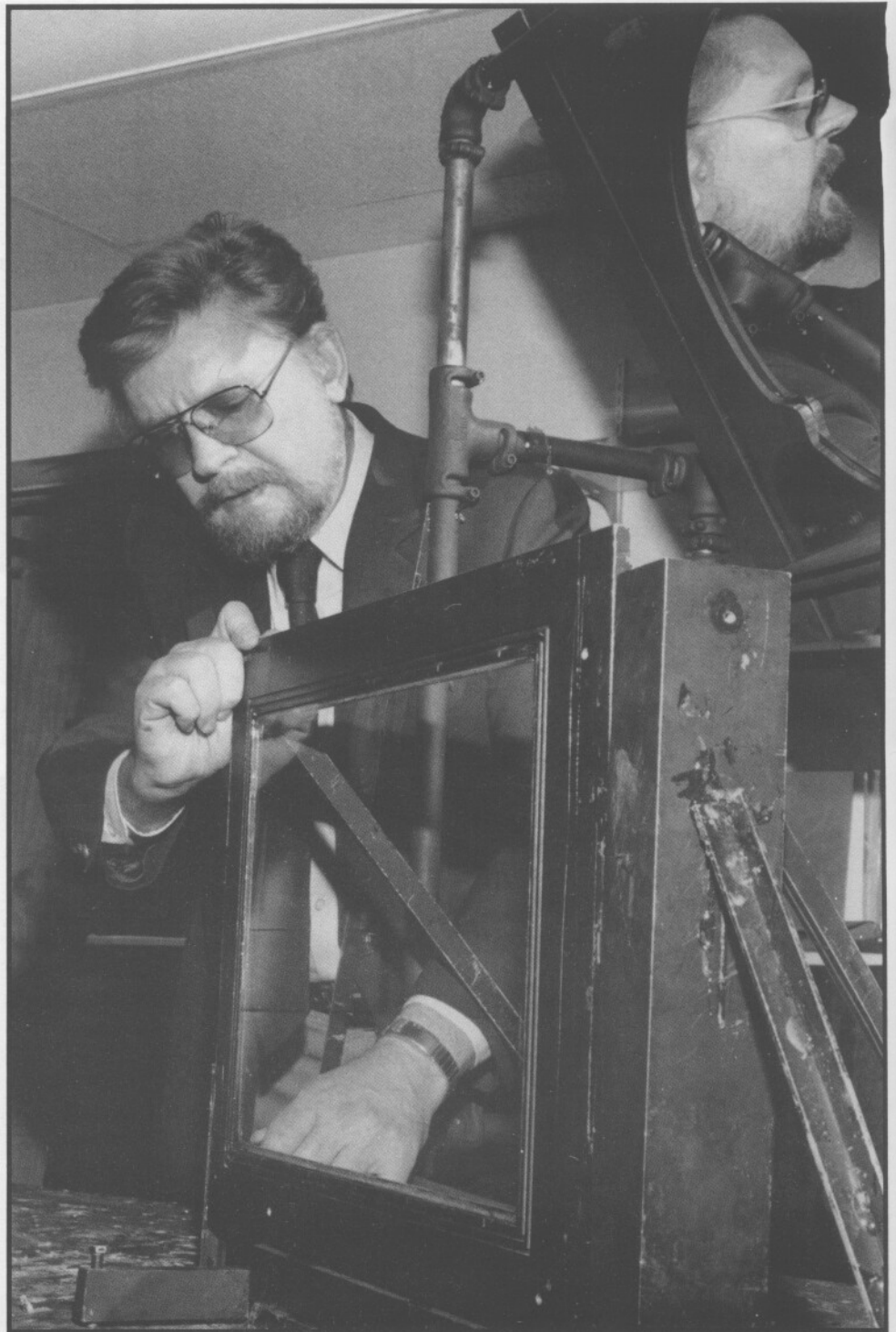
Rudolph Guzik, president, Imaging Technology Consultants, checks vacuum plenum on large format film holder during setup of non-destructive test
