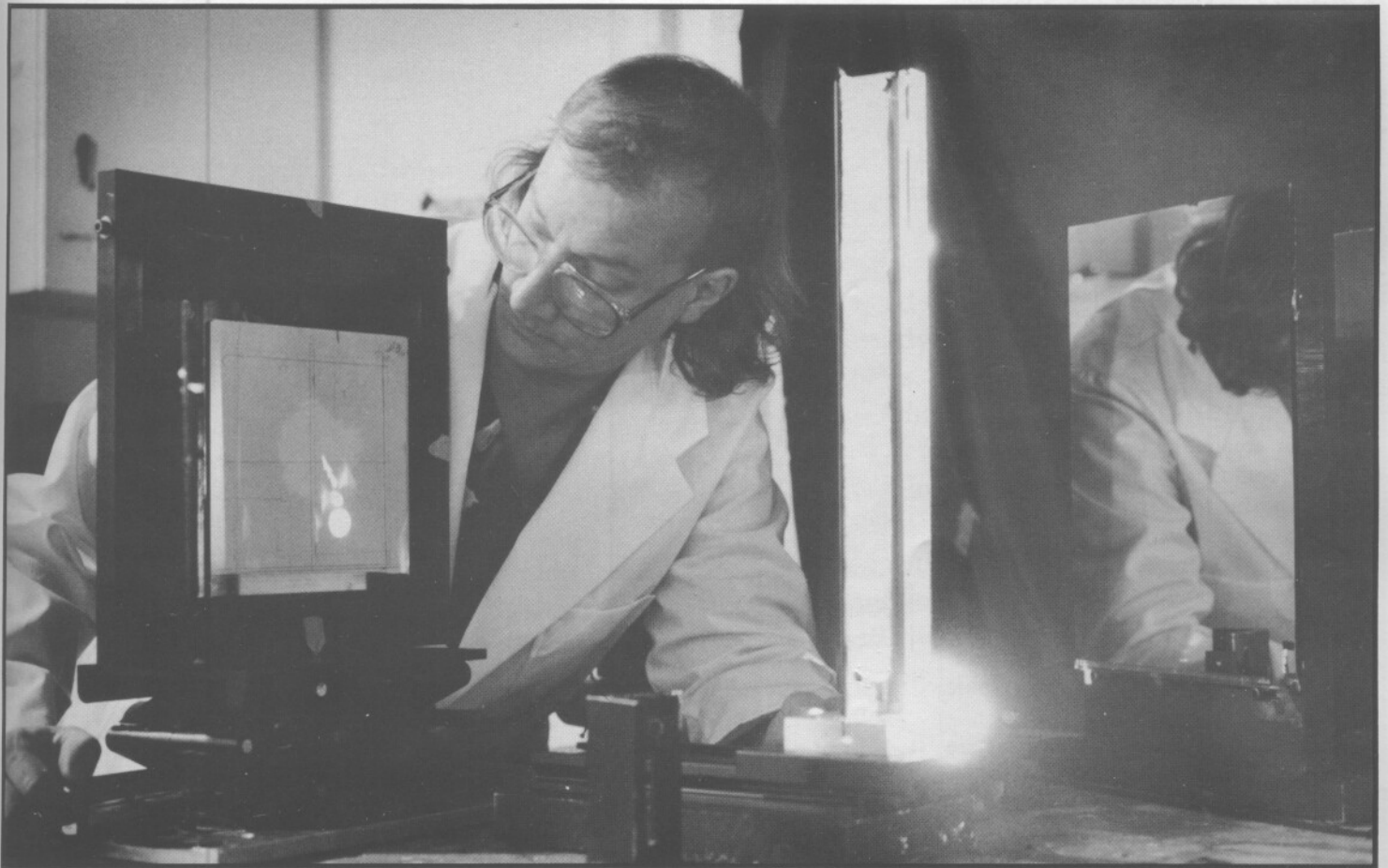
Steve Smith aligns the film holder for the focused image rainbow hologram
